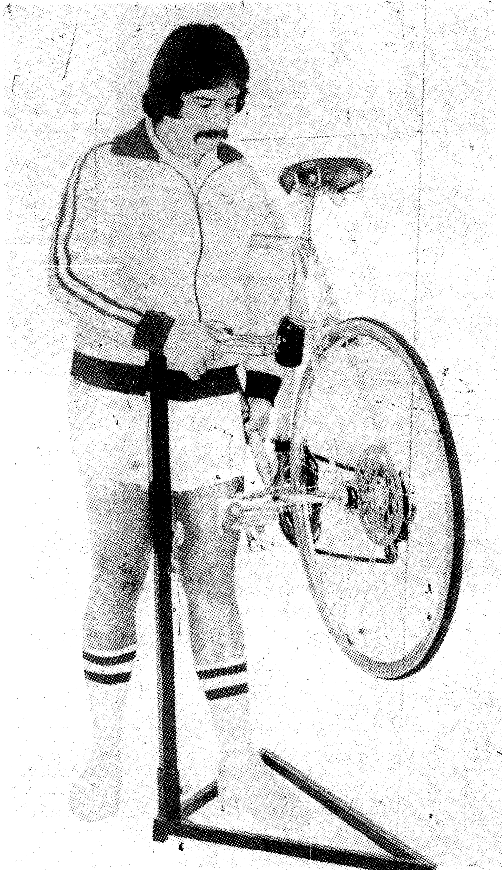
Fig. 4-5. Clamping a bike on a stand.
