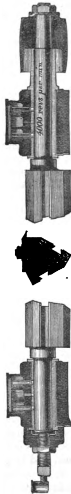
Fig. 14.—Cutter Block and Spindle for 14-in. trying-up Machine.
